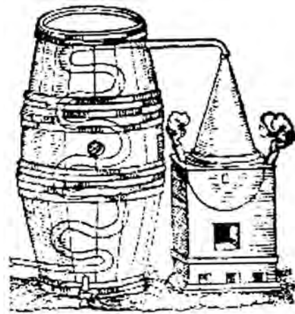
A still with worm and worm tub, from an engraving made in 1551. This is the first known illustration of this apparatus.
